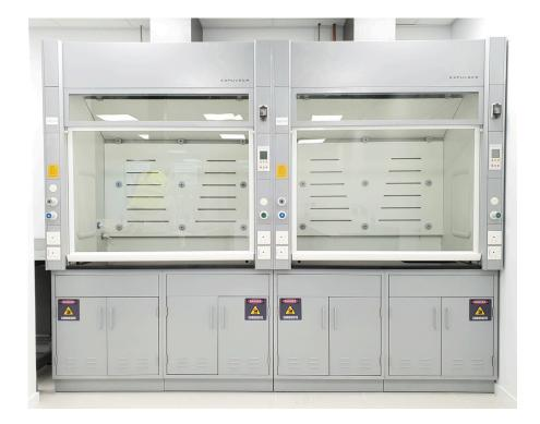
A Laboratory fume hood (Fume cupboard) is a type of local exhaust ventilation system inside the laboratory. It is a typical enclosed cabinet except front face. The front opening will be equipped with a moving sash made out of toughened / safety glass. Air is drawn in to the hood under, through the opened sash and is exhausted through openings in the rear & top of the cabinet to a remote point such as an exhaust stack on the roof of the building.
